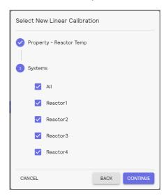
The user can then complete a two-point calibration, with one high and one low value. When entering one of these values, the stability of the value is displayed to help the end-user know when it's appropriate to calibrate the sensor.
