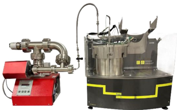
Figure 1. H.E.L's BTC-130 attached to a mass spectrometer.
